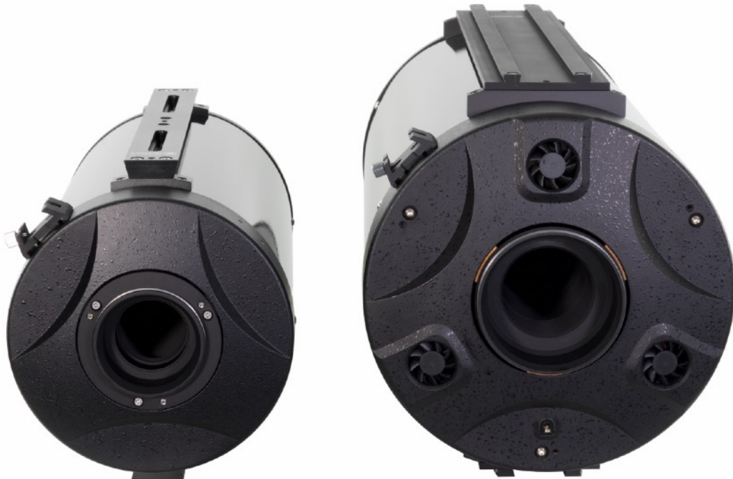
ESATTO as focuser for Ritchey-Chretien telescopes: to the left the 90mm thread that you can find on GSO 6" or 8" Ritchey-Chretien telescopes. To the right, the 117mm thread that you can find on GSO 10", 12", 14" or 16" Ritchey-Chretien telescopes.
