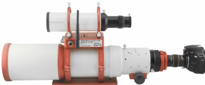
Nikon DSLR camera connected with projection (with 3x Barlow lens) to apochromatic refractor: this way we use it at 650mm x 3 = 1950mm focal length (f18.75)
