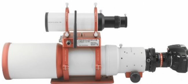
Nikon DSLR camera connected in prime focus (with field flattener) to apochromatic refractor: this way it uses the telescope as a 650mm (f6.25) telephoto lens
